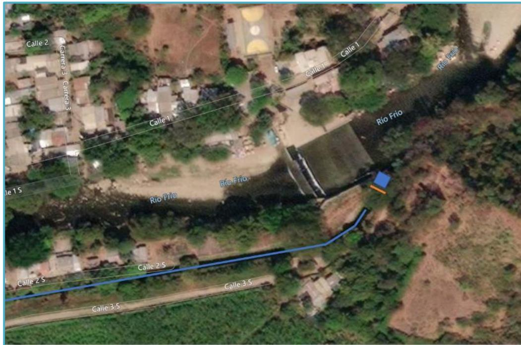
Figure 4-3. The Río Frío, at the village Río Frío, and the primary water infrastructures of ASORÍOFRIO, with the main intake (blue square), the weir structure (orange line), and canal Santa Inés (blue line), in zoom below, Bing maps Imagery.
