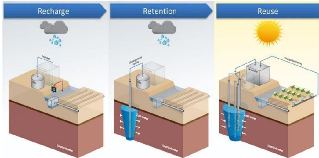
Figure 50. An example of an Aquifer Storage and Recovery(ASR) system. Image of Acacia Water.
