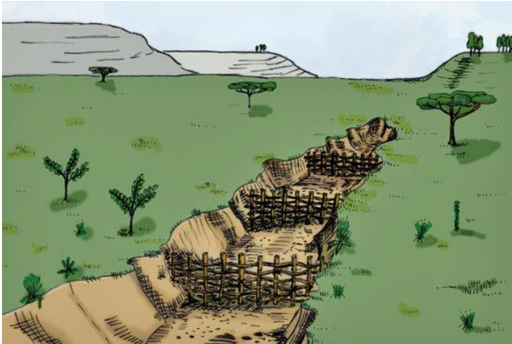
Figure 19. Sketch of a gully treated with a check dam, which in this case consists of brushwood. This can be very effective, particularly for smaller gullies, which are refilled with soil over a longer period. Instead of brushwood also hardcore boulders and/or bamboo shoots can be used. The structures should not be too far apart (source: Hurni et al., 2016).
