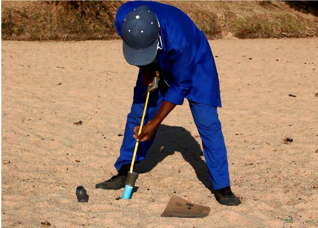
Figure 5. Mr. Lisani Mathanda recording groundwater levels from a piezometer at ALL ONE irrigation scheme, July 2020. Photo; Celine Muzarabani
