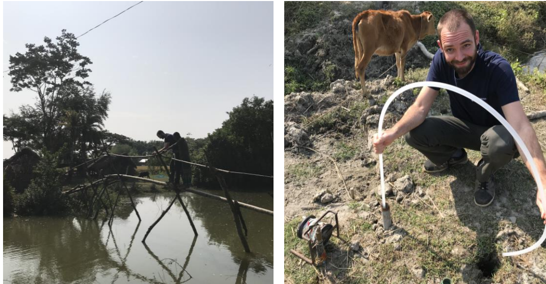
Figure 18. Photo of the EC measurement from the bridge in the middle of the river (left) and sampling of water from the exploration borehole (RAF-2) by means of an inertial pump with ball-valve
