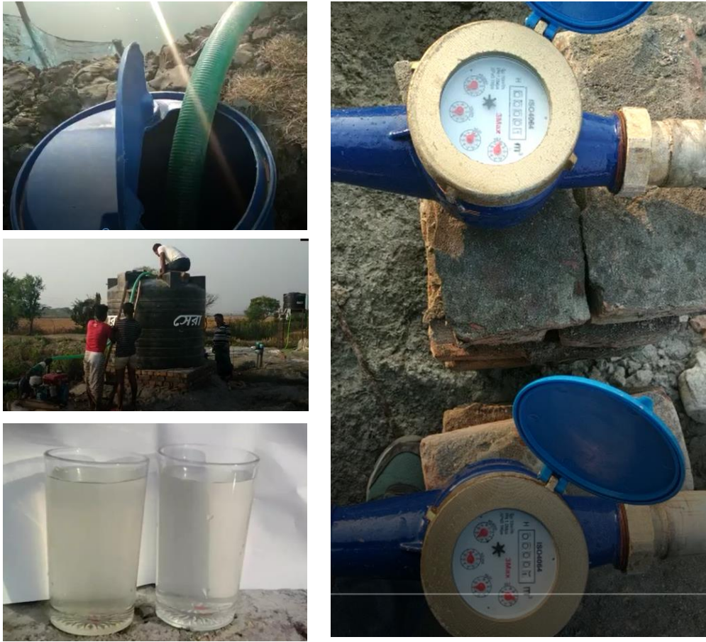
Figure 21. Photos of the testing of the AgriMAR system, showing the flow meters of the infiltration of the shallow and deep filter screen (right), the water being pumped from the drain via the collector tank (upper left), filling of the 5000 liter PE reservoir (middle left), and comparing the higher turbidity of the pond water with the filtered water (lower left)
