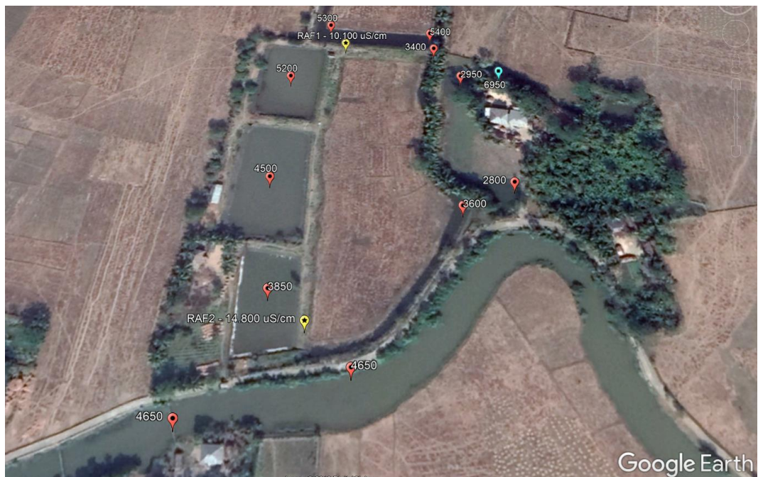
Figure 19. EC measurements at and around the AgriMAR site in December 2018.
