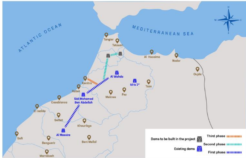
Figure 4-14. The planned water transfer (Source: El Mocayd et al. , 2019). Project implementation is ongoing. The proposed north-south water transfer project (Water Highway) aims to supply water to the arid southern regions from the watersheds in the north.
